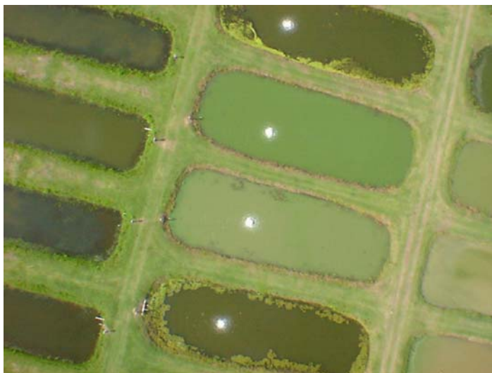
Figure 2.3: Digital photograph of aquaculture ponds taken from autonomous airplane shows different visual characteristics of ponds, which can be linked to water quality and algae growth in ponds for improved management of aquacultural operations (Photo by R. Price).
