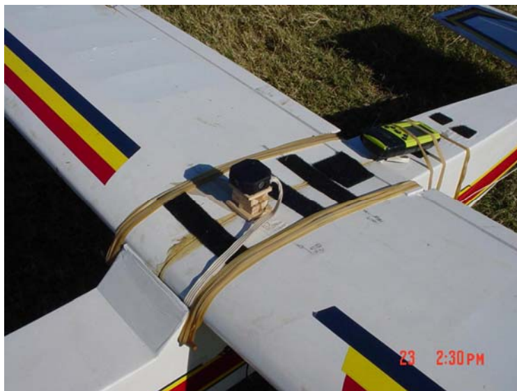
Figure 2.2: Photograph of semi-autonomous airplane shows self leveling horizon finder (black, center); and GPS (yellow and black/toward rear of plane). Microelectronics and associated control hardware (e.g. servos) are enclosed primarily in center of airplane. A digital camera was mounted in the lower part of the airplane viewing downward (Figure2.3; Photo by R. Price).
