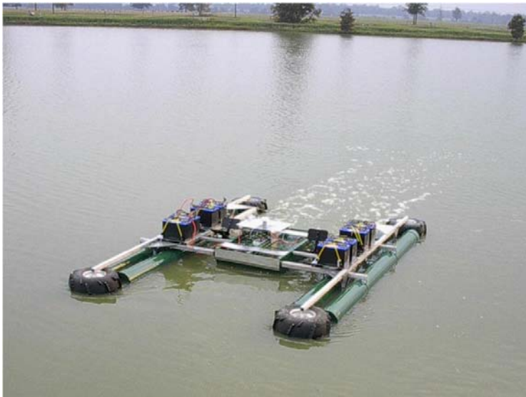
Figure 2.1: One version of a series of autonomous boats developed in the Department of Biological and Agricultural Engineering of the LSU AgCenter, here being tested at the LSU AgCenter Aquaculture Research Station in Baton Rouge, Louisiana, USA. This one was large (3x4m, 500kg), and intended to reduce bird incursions on large (e.g. 10-1000 ha) aquaculture ponds and/or drinking water reservoirs. The basic organization still included solar power (not shown); batteries; paddlewheels; microcontrollers and GPS guidance.
