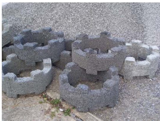
Figure 3.3: A photograph of both interlocking rings and bars with encased oysters reveals the desired texture: capable of providing refuge for young oysters and good reduction of wave energy, while locking or stacking together.
