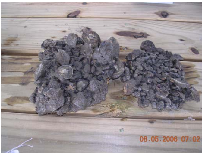
Figure 3.5: Growth of oysters shows further enhancement of the porous interlocking structure which allows for habitat as well as wave energy reduction.
