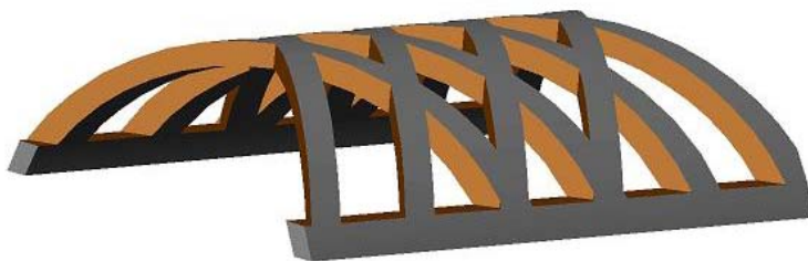
Figure 4.1: The engineered reef design shown requires 80% less material than a solid reef; provides habitat and surface area for reef builders such as oyster or coral to grow, and is much lighter than solid materials, reducing cost and enabling quick emplacement.
