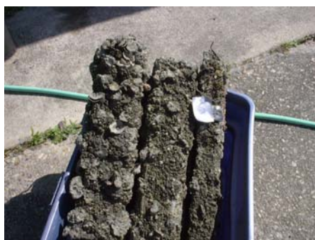
Figure 3.4: Growth observed on biologically enhanced engineered bars after approximately 4 months of growth suggests annual growth rates in the range of 5-10 cm, with 2-4 layers of interlocking oysters cementing components together.
